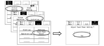
Press the center of the X mark, then the position of the mark changes one after another. Press five marks sequentially.
