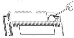
(5) Put a new replacement battery into the battery holder.
