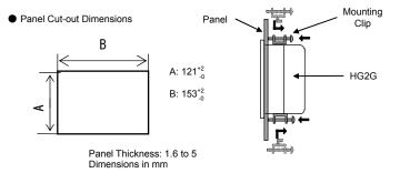
Place the HG2G in a panel cut-out and fasten with the attached mounting clips at four places to a specified torque of 0.12 to 0.17 N·m uniformly.
