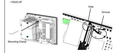
Procedure 6. Fasten the mounting clamp with the screw to a specified torque of 0.6 N·m pushing the mounting clamp as shown in the following figure. After fastening the mounting clamp, make sure that the mounting clamp is not loose and not having a gap.
