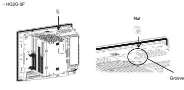
Procedure 5. Insert the A side of the mounting clamp into the groove. And hook the B side of the mounting clamp on the hole of the expansion module.
