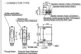
Note1: Stability Indicator and Sensitivity Control and Operation Mode Switch are not attached to the Emitter of Through-Beam Type.
