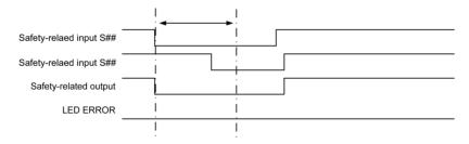
Both safety-related inputs are deactivated within the signal interlock monitoring time of 200 ms. When they are activated again, the safety-related outputs are also activated.
