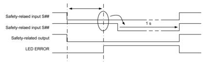
The first safety-related input is deactivated which starts the signal interlock monitoring time of 200 ms. The second safety-related remains activated longer than 200 ms. This triggers a signal interlock alert 200 ms after interlock monitoring has started.
