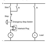
Note 1: When using the main circuit on AC, connect emergency stop switch to Line, and interlock plug unit to Neutral.
