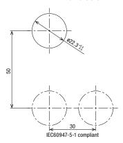
Determine mounting centers to ensure easy operation.
