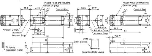
Note: Plug the unused actuator insertion slot using the slot plug supplied with the interlock switch.
