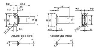
**Actuator Mounting Hole Layout** (Straight, Right-angle)
