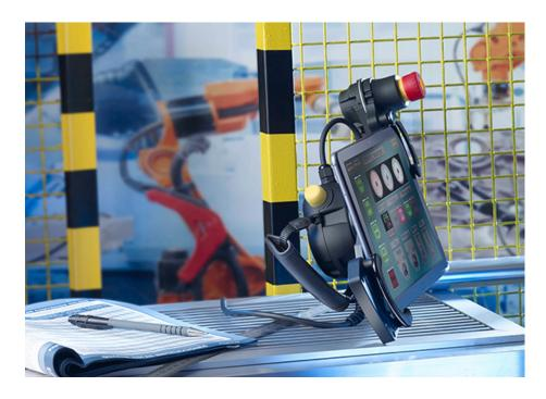
IDEC's innovative HT3P Safety Commander™ easily and affordably turns any standard tablet into a rugged control terminal with a easy-to-use touch panel and all the standard-compliant safety features required for industrial applications.
