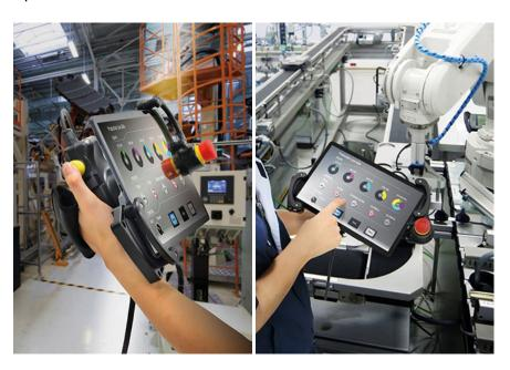
Thanks to the integrated IDEC enabling and emergency stop switches, the HT3P Safety Commander™ provides for both ergonomic operation and controlling of industrial systems and devices that is safe at all times.
